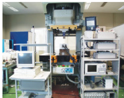
Fig. 7 Experimental apparatus of the experimental analysis system to visualize inner stress of a die
